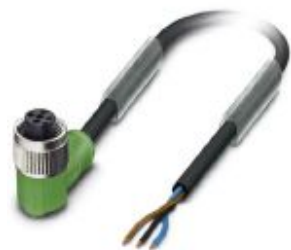
Sensor/actuator cable, 3-position, PUR halogen-free, black-gray RAL 7021, free cable end, on Socket angled M12, coding: A, cable length: 1.5 m
