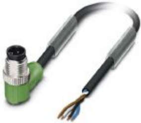
Sensor/actuator cable, 4-position, PUR halogen-free, black-gray RAL 7021, Plug angled M12, coding: A, on free cable end, cable length: 10 m
