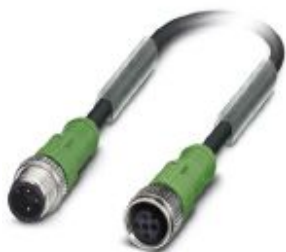
Sensor/actuator cable, 3-position, PUR halogen-free, black-gray RAL 7021, Plug straight M12, coding: A, on Socket straight M12, coding: A, cable length: 10 m
