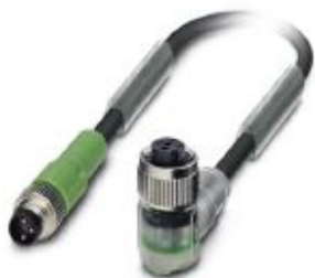
Sensor/actuator cable, 3-position, PUR halogen-free, black-gray RAL 7021, Plug straight M8, on Socket angled M12, coding: A, with 2 LEDs, cable length: 3 m
