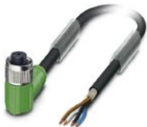
Sensor/actuator cable, 4-position, PUR halogen-free, black-gray RAL 7021, shielded, free cable end, on Socket angled M12, coding: A, cable length: 3 m
