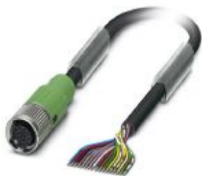
Sensor/actuator cable, 17-position, PVC, black RAL 9005, free cable end, on Socket straight M12 SPEEDCON, coding: A, cable length: 15 m
