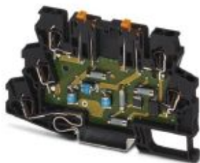
TERMITRAB, spring-cage modular terminal block with integrated surge protection and disconnect knives, for assembly on NS 35/7.5, voltage U_N 24 V DC, terminal width: 6.2 mm, cover width: 2.2 mm
