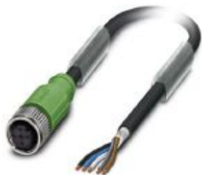
Sensor/actuator cable, 5-position, PUR halogen-free, black-gray RAL 7021, shielded, free cable end, on Socket straight M12, coding: A, cable length: 3 m
