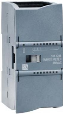
SIMATIC S7-1200, Analog input, SM 1238 Energy Meter 480 V AC, power measurement module for data acquisition in 1- and 3-phase supply systems (TN, TT) up to 480 V AC; Current range: 1 A, 5A; acquisition of voltage, current, phase angles, power, energy values, frequencies; Channel diagnostics
