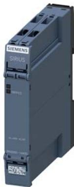
Thermistor motor protection relay Compact evaluation unit, 17.5 mm enclosure, screw terminals, 1 changeover contact, US = 24 V-240 V AC/DC, Auto RESET, suitable for bimetallic switch, supply =output voltage, 1 LED (tripped)
