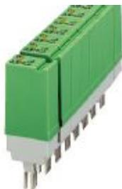
Plug-in power solid-state relay, with LED and protective circuit in input and output circuits, input: 24 V DC, output: 12 - 60 V DC/max. 3 A, can be plugged into basic terminal blocks
