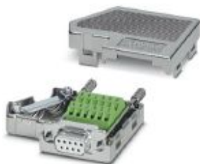
D-SUB connector, 9-pos. female connector, two cable entries < 35°, bus system: CANopen, FIP, pin assignment: 2, 3, 6, 7, 8, 9 to two screw connection terminal blocks
