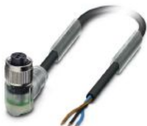
Sensor/actuator cable, 3-position, PUR halogen-free, black-gray RAL 7021, free cable end, on Socket angled M12, coding: A, with 2 LEDs, cable length: 3 m
