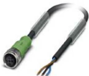
Sensor/actuator cable, 3-position, PUR halogen-free, black-gray RAL 7021, free cable end, on Socket straight M12, coding: A, cable length: 5 m
