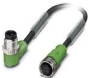
Sensor/actuator cable, 4-position, PUR halogen-free, black-gray RAL 7021, Plug angled M12, coding: A, on Socket straight M12, coding: A, cable length: 0.6 m
