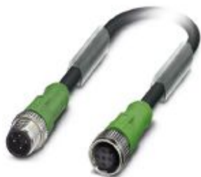
Sensor/actuator cable, 4-position, PUR, black-gray RAL 7021, Plug straight M12, coding: A, on Socket straight M12, coding: A, cable length: 2 m
