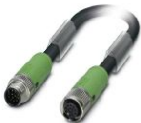
Sensor/actuator cable, 12-position, PUR/PVC, black RAL 9005, shielded, Plug straight M12 SPEEDCON, coding: A, on Socket straight M12 SPEEDCON, coding: A, cable length: 3 m
