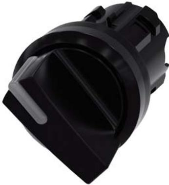
Illuminable selector switch, 22 mm, round, plastic, black, Selector switch short, 2 switch positions O<I, momentary contact type, Actuating angle 45°, 10:30h/12h
