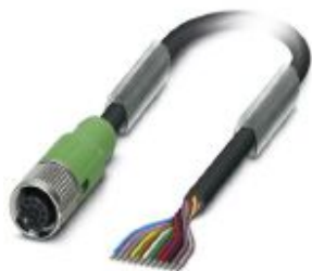
Sensor/actuator cable, 12-position, PUR halogen-free, black RAL 9005, free cable end, on Socket straight M12 SPEEDCON, coding: A, cable length: 10 m
